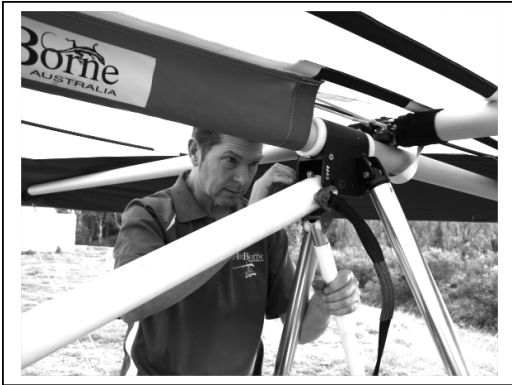
Figure 15 Section 4. Attach Wing to Wing U-Bracket
