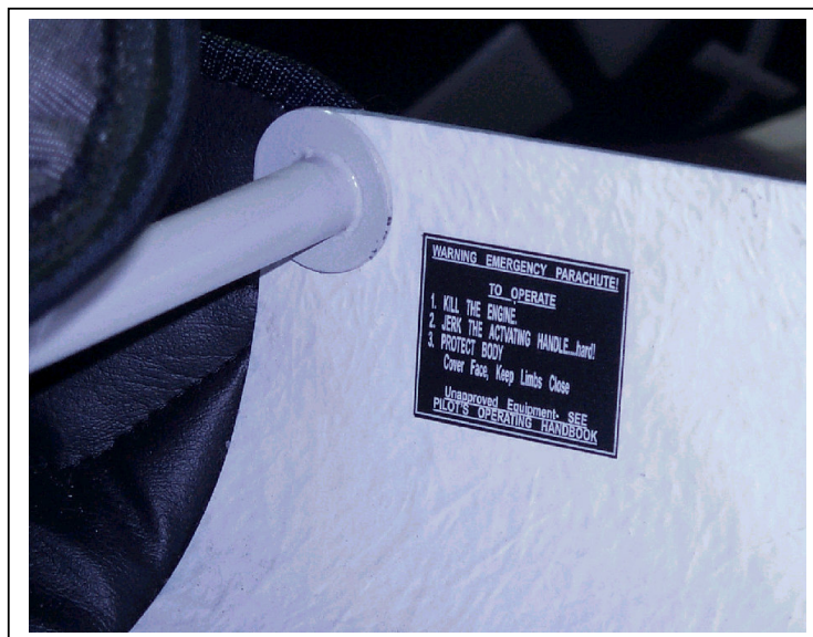
Figure 19 Section 2. Parachute Placard Location – (Pilots Left on Pod near to Seat Frame)
