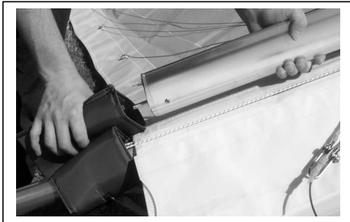
Figure 32 Section 4. Remove King Post
