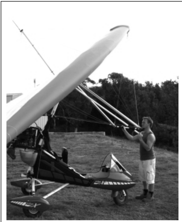
Figure 21 Low Hangar Position
