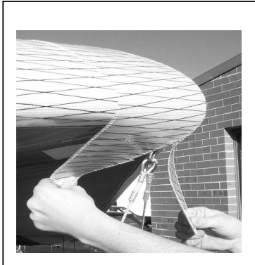
Figure 10 Section 4. Install Nose Fairing
