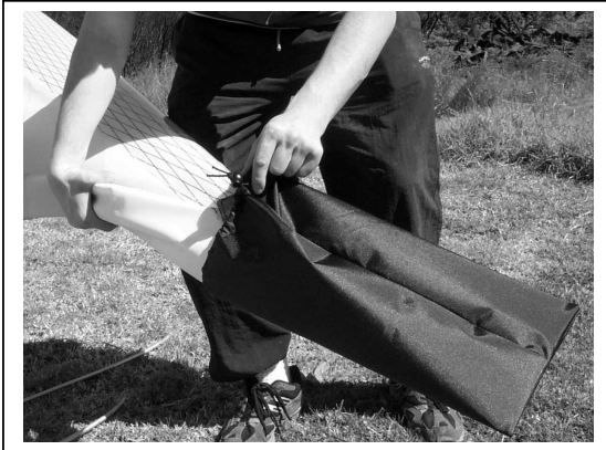
Figure 25 Section 4. Fit Tip Bags
